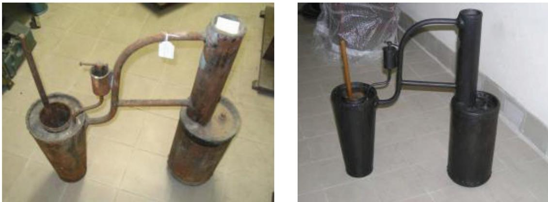
Figs. 8 and 9: Ferdinand Carré's apparatus, before and after restoration, MCUL 2035
